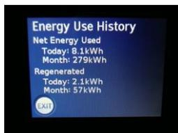
*Car 1 used 279 kWh over May, 350 after losses. Note 57 kWh of regen. added range.*
