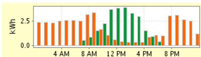
Size & shape of our solar *made* (in green) above is predictable – roughly a parabola from around 8 am through 6 pm and this matches (no surprise!) sunshine. These are hours very usefully too a Utility values power most dearly. Of course PV *production* (green) didn't change at all when this car 1 was added at one-side of the PV+EV equation.
