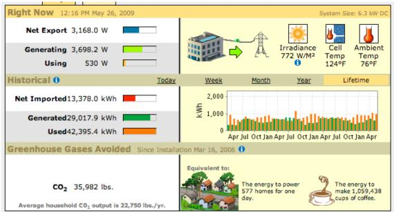
29,000 kWh was generated & measured since a  $2^{nd}$  PV monitoring was installed in 2006 (left). For this sample sunny On-peak moment (left, top), Irradiance is a sunny 772 W/M<sup>2</sup>; our PV is making 3,698 Watts, demand that moment is 530 Watts, and 3,167 Watts is being exported.
